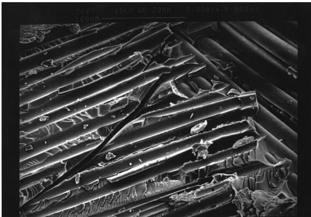
Figure 12 WMG Random Continuous Glass/Epoxy Laminates with 41.2% fibre volume fraction showing crack running through debonded matrix ( \times 366 ).
