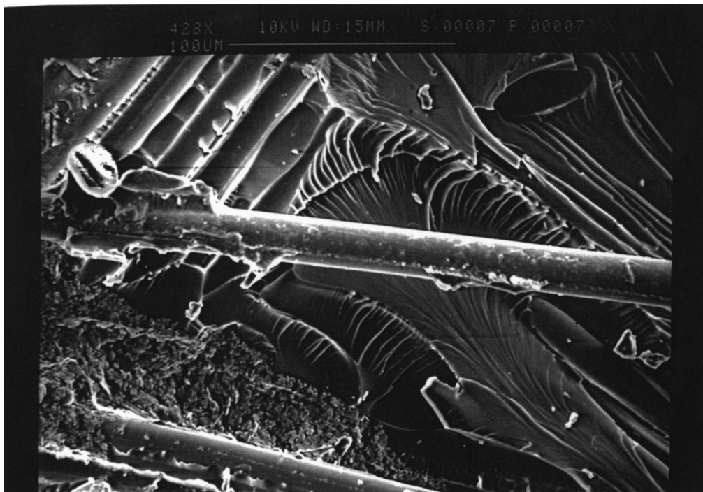
Figure 6 WMG Random Continuous Glass/Epoxy Laminates with 20.7% fibre volume fraction showing areas of fibre-matrix adhesion, fibre pull-out and fibre-matrix debonding ( \times 428 ).
